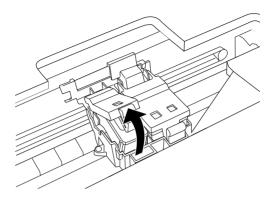
5. Take out the cartridge and then dispose of it properly. Do not take the used cartridge apart or try to refill it.
